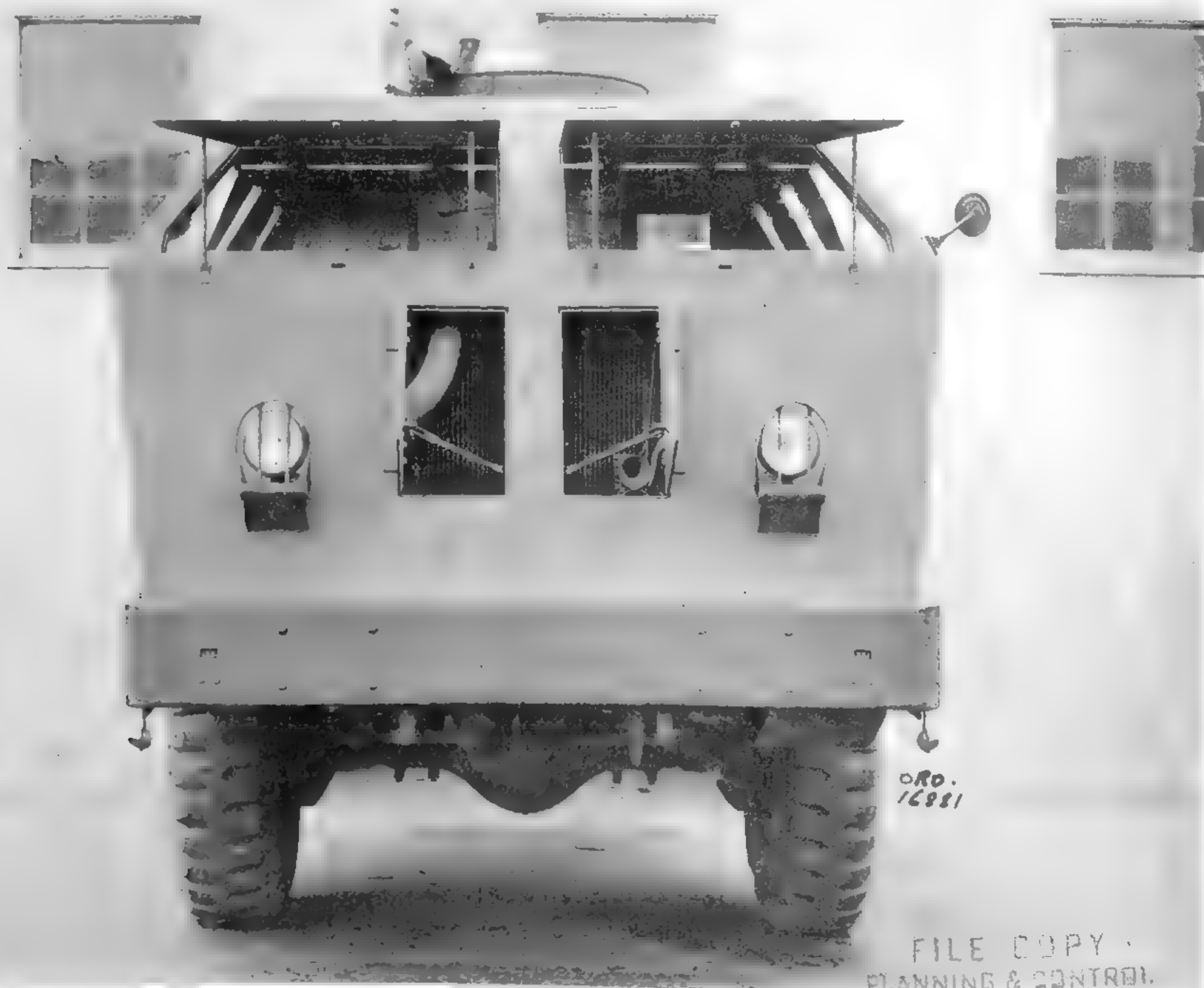
This front view is of the prototype M26 built by the Knuckey Truck Company. While the basic design had been worked out, there was some refinement before the vehicles were mass produced. (U.S. Army photo)
